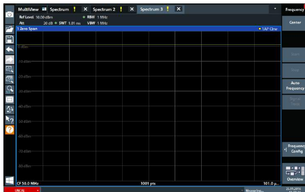
Figure 4-10: Time domain display of the calibration signal
