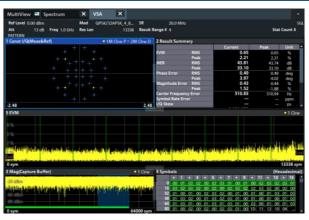
$\label{lem:lemodulation} Demodulation of a DVB-SX2\ multi-modulation\ signal\ with\ the $R\&S^*FPL1-K70M\ option\ (R\&S^*FPL1-K70\ option\ required).$
