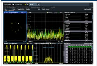
Analysis of a Bluetooth 3-DH1 signal. Constellation diagram, EVM, result summary, magnitude, spectrum and symbols with pattern detection all in one view.
