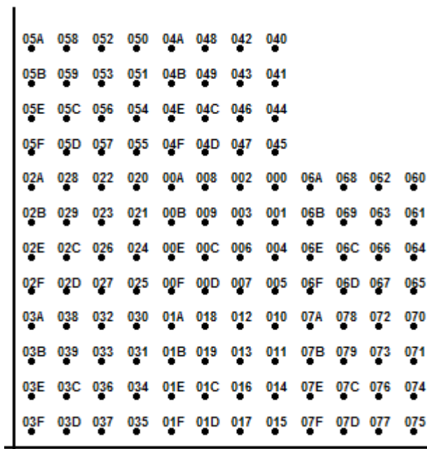
Figure 4-46: Constellation diagram for 512QAM (NATURAL, SMx), including the logical symbol mapping (hexadecimal); the figure shows the upper right section of the diagram only
