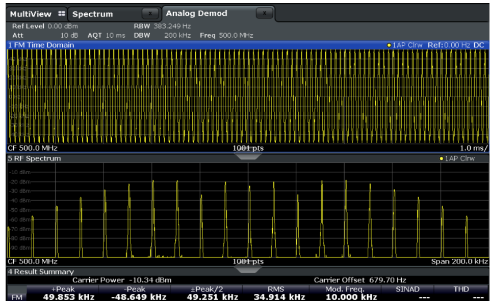
Figure 9-5: RF spectrum with demodulation bandwidth = 200 kHz
