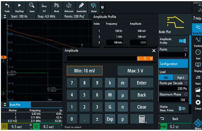
The amplitude output level of the generator signal can be varied during the measurement to suppress the noise behavior of the DUT
