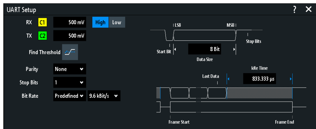
Figure 12-18: UART setup dialog
