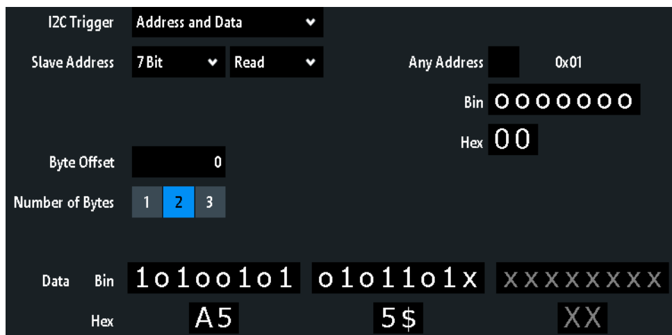
Figure 12-13: Trigger setup dialog to trigger on a combination of address and data
