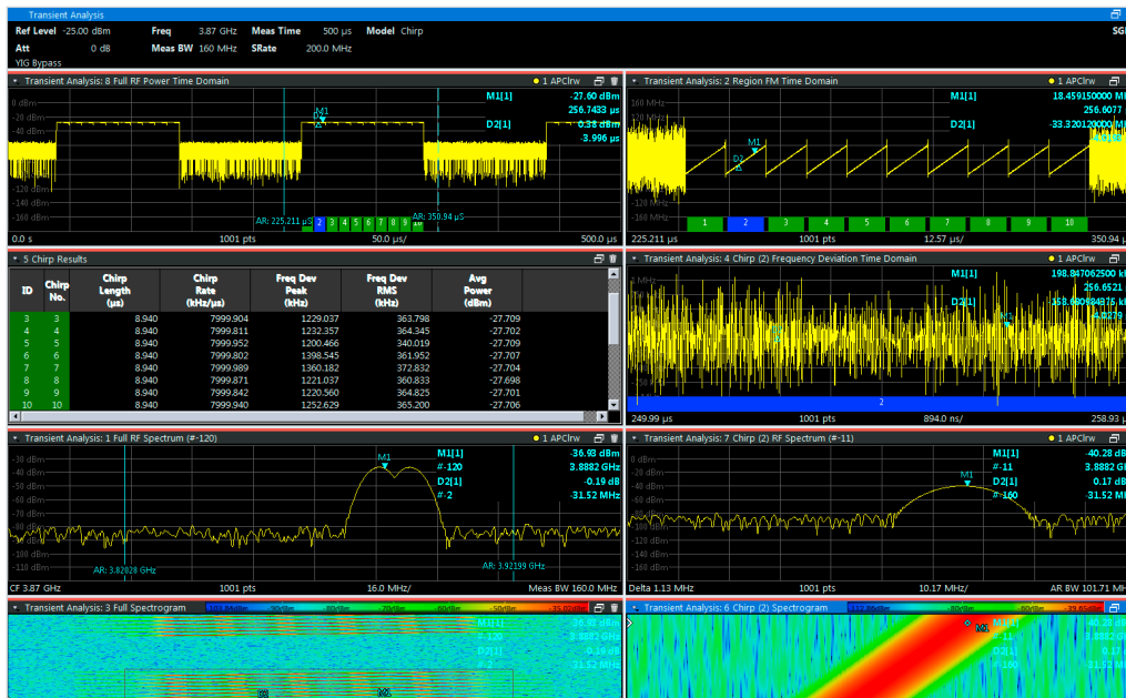
Analysis of a chirp signal with different measurement windows
