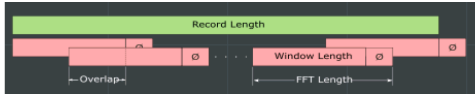
Figure 10-2: FFT parameters for averaged FFT calculation
