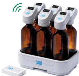
RESPIROMETRIC Sensor System - BOD 6 positions - Results on display and RESPIROSoft™
