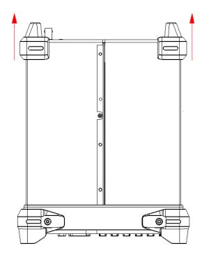
4. Remove the screw on the bottom of the instrument and place it in a safe location for re-assembly. Slide off the instrument cover as indicated by the arrow shown below.
