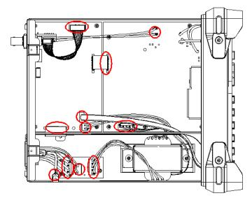
6. Unscrew the 5 captive screws in the rear metal cover and remove the rear metal cover.
