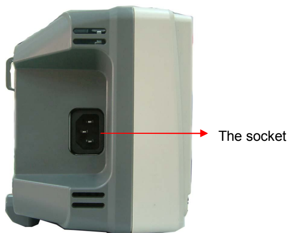
Figure 2-1 Connect power line
