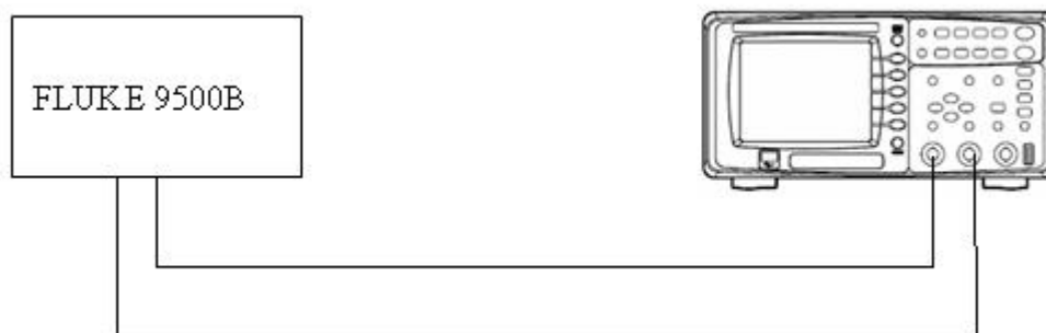
Picture 3-1 Connecting test instruments
