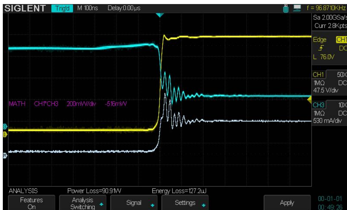
Figure 121 Perform Switching Analysis
