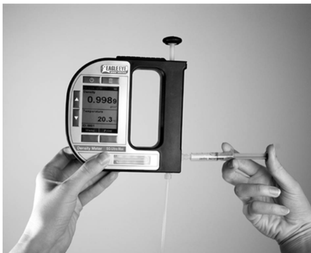
Fig. 10 - 2 Filling sample using the plastic syringe
