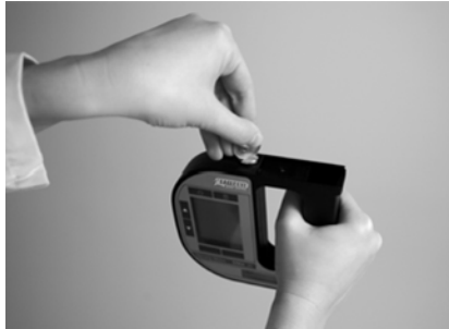
Fig. 12 - 4 Opening the battery cover
