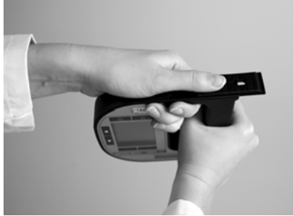
Fig. 12 - 3 Removing the pump lock
