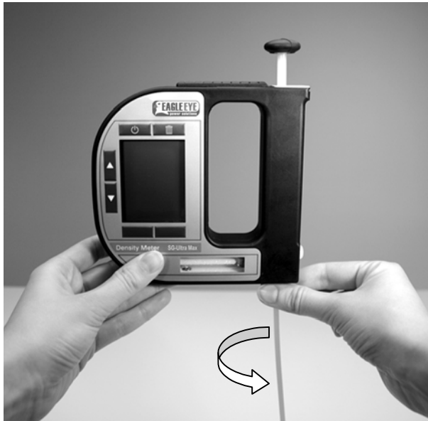
Fig. 7 - 1 Connecting the filling tube
