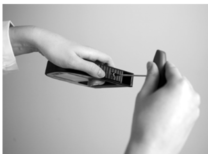
Fig. 12 - 2 Removing the pump lock screw
