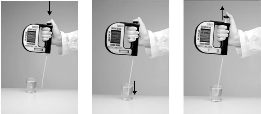
Fig. 10 - 1 Filling sample using the filling tube
