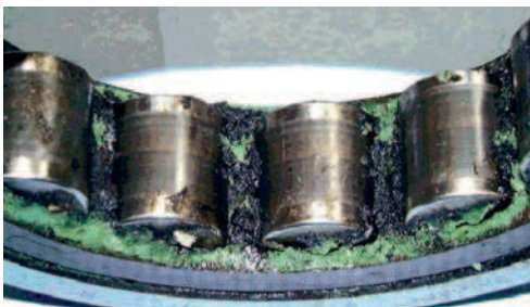
Lubricant degradation caused by electrical discharge currents
