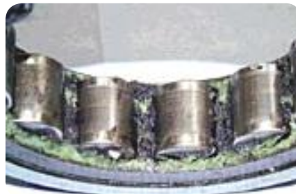
Lubricant degradation caused by electrical discharge currents.
