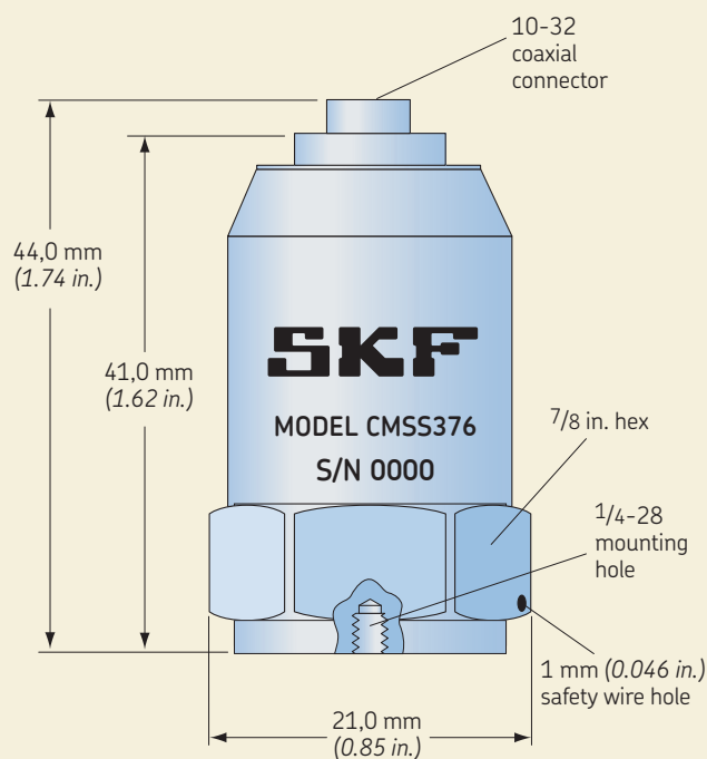
CMSS 376 accelerometer dimensions
