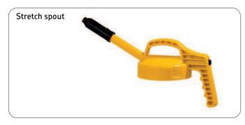
Ideal for precise pouring tasks and areas that are difficult to access. The 12 mm (0.48 in) outlet is ideal for viscosities up to ISO VG 220.
