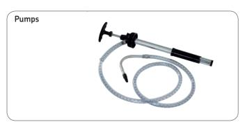
Standard pump suitable for viscosities up to ISO VG 460. High flow (approx. 14 strokes per litre/US quart). High viscosity pump for viscosities up to ISO VG 680. High efficiency with approx. 12 strokes per litre/US quart. As a protection against airborne contaminants during the pumping process, a 10 micron breather is available. For both pumps an anti-drip long discharge hose of 1.5m (4.9 ft) and reducer nozzles are available.
