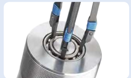
The springs enable easy insertion
