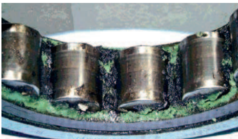
Lubricant degradation caused by electrical discharge currents
