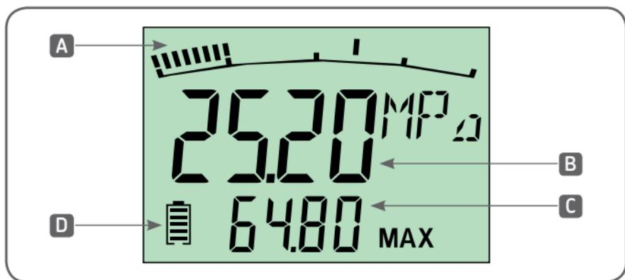
The actual pressure is indicated in the display mode. The measured value is displayed in the corresponding unit. The MAX or FS value is indicated in the lower part of the display.
