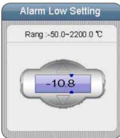
Press the ENTER button on the first row and use the UP and DOWN button to adjust value. Press the ENTER button to confirm, press the ESC button to esc and save.
