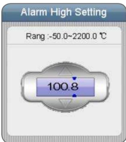
Press the ENTER button on the first row and use the UP and DOWN button to adjust the value. Press the ENTER button to confirm, press the ESC button to esc and save.
