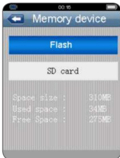
Press the UP and DOWN button to select the Memory device, press the ENTER button to enter. The internal memory or the memory card can be selected.
