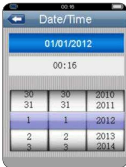
Press the UP and DOWN button to select the date or time, then press the ENTER button to enter, press the UP and DOWN button to adjust the value, press the ESC button to esc and save.
