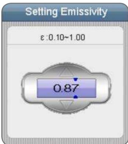
ON the first Item, press the ENTER button to adjust emissivity, press the UP and DOWN button to adjust the value, then press the ENTER button to confirm. Press the UP and DOWN button to select the emissivities of the materials, press the ESC button to esc and save.
