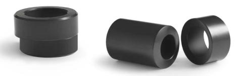
Spherical washers from SKF are designed to create an exact parallel plane between the bolt head and the face of the nut. This spherical washer automatically adjusts to compensate for angle errors and eliminate bolt bending.
