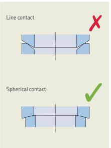
Industrial spherical washers (DIN) consist of a conical ring and a spherical ring resulting in a line contact with a limited load capacity. SKF Spherical Washers consist of convex and concave rings to create a perfect mating surface and have a high load bearing capacity as result.
