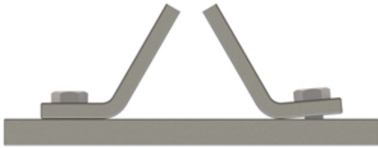
Angular soft foot: bent foot
