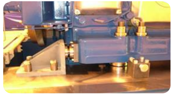
In addition to its functionality as a chock, the SKF Vibracon can also be used as a stopper.
