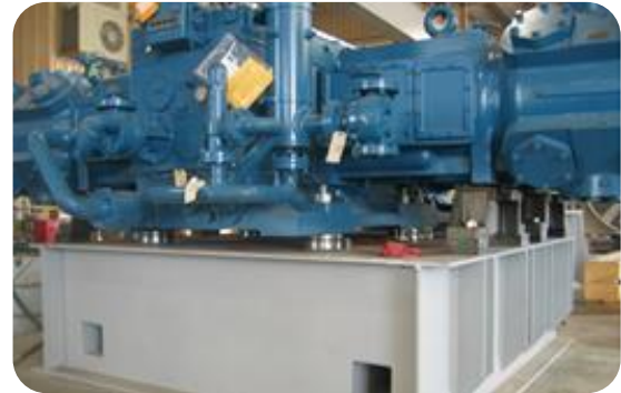
Re-adjustable fixed point to avoid reaming of fitted bolt holes.
