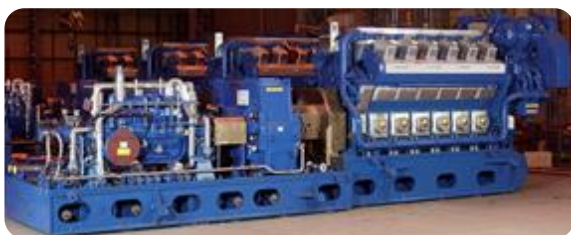
Crude oil pump set, engine and gearbox mounted on SKF Vibracon chock.
