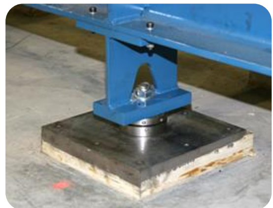
Chocking of the structure
