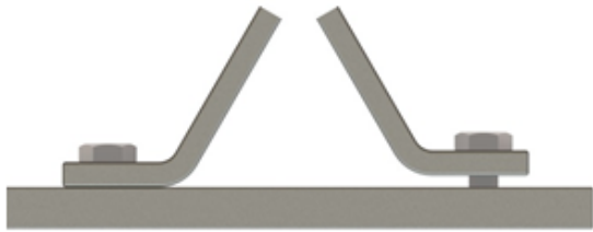
Parallel soft foot: short foot
