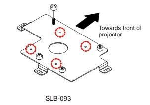
(Note: SSB-style interface bracket connections are encircled)
