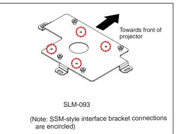
NOTE: Specific to SSB-style and SSM-style interface bracket installation, all appropriate screws come pre-installed as reflected in the encircled locations above. DO NOT attempt to substitute and USE ONLY this pre-installed hardware for SSB-style and SSM-style interface bracket installation.
