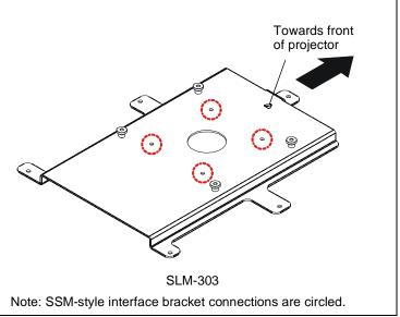
**NOTE:** Specific to SSB-style and SSM-style interface bracket installation: All appropriate screws come pre-installed in the circled locations above. DO NOT attempt to substitute and USE ONLY this pre-installed hardware for SSB-style and SSM-style interface bracket installation.
