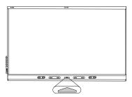
Press the **Home** button on the display (pictured) or the remote control to open the Home screen. From the Home screen, you can open the iQ apps, switch inputs, and adjust settings.
