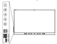
The convenience panel provides buttons for turning the display on and off, controlling the volume, freezing and unfreezing the screen, and showing and hiding a screen shade. It also includes connectors for USB peripherals and a computer or other input source.
