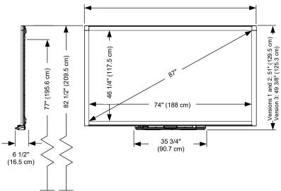
Leave at least 5/8" (1.6 cm) headroom to wall mount the SB885. The distance from the bottom of the wall mount bracket to the top of an installed interactive whiteboard is 6 1/8" (15.6 cm)
