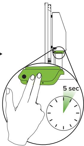
Press and hold the control switch for 5 seconds.
