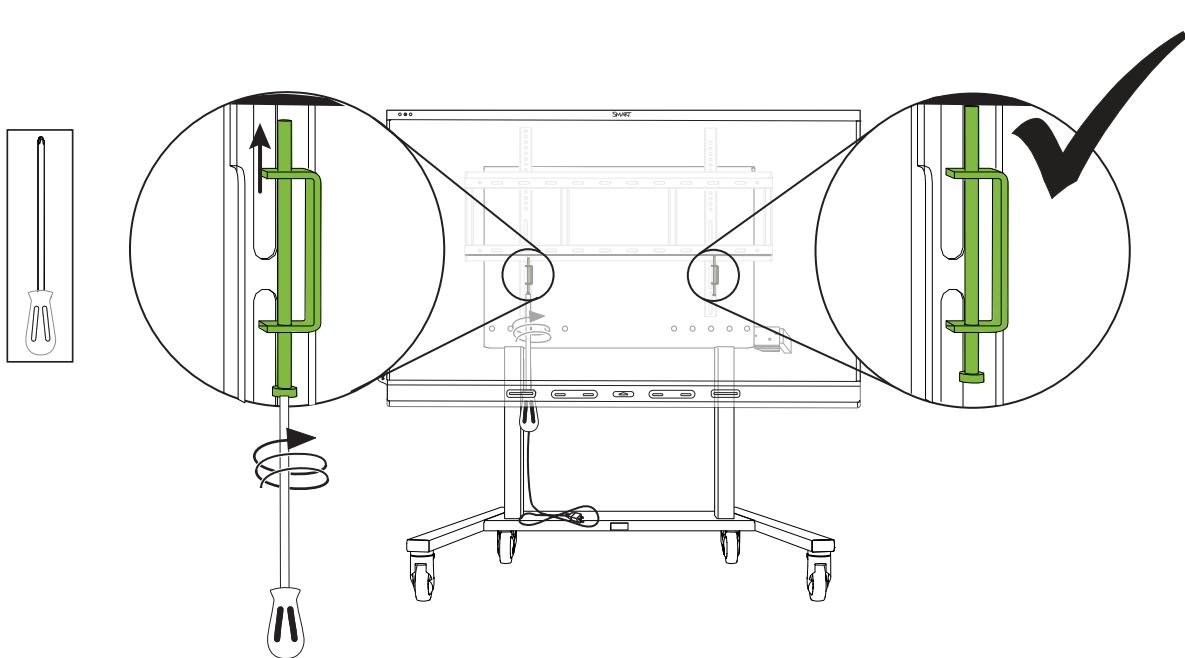
Secure the display to the wall plate by tightening the locking screws with a Phillips No. 2 screw driver until the screws contact the wall plate.
