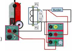
10. CT, Voltage method: Calculates the CT turn ratio and polarity, by injecting Voltage, for the cases where is not possible to directly inject primary current into the CT, for whatever reason, being this template an alternative. Disconnecting the load, it is performed applying voltage on its secondary side with the auxiliary output of Raptor, and measuring the secondary voltage with the voltmeter and the primary voltage with the low signal voltmeter.
