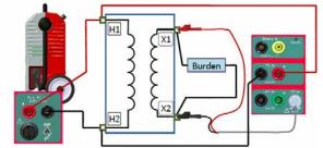
**12. VT burden:** Calculate impedance, power and power factor of the load, disconnecting the secondary of the VT, and applying voltage to the load from the auxiliary voltage output of Raptor, and measuring with the ammeter and voltmeter.
