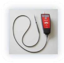
**15. Polarity Test:** Specific template to be used with the optional accessory Raptor Polarity Tester (Raptor PT), to check polarity and correct wiring of all secondary circuits, while the Raptor is injecting a special polarized signal from the primary of the transformers.
