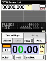
**Pulses Train:** This function allows the generation of pulses at regular intervals, with the setting of the injection time and off time between pulses. It is possible to use any of the output sources of the Raptor (high current, low current, low voltage or high voltage with HV).
