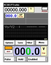
**14. PT ratio:** Measures the voltage ratio between the primary winding and the relative secondary winding of a PT. If the PT is three-phase, a measurement must carry out in each phase. If the neutral is not accessible in either of the two windings, inject between two phases (H1H2) and measure on the Low side in agreement with the calculation and connection diagram required, depending on the PT connection group.
