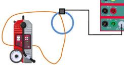
7. AC resistance: measures the resistance of connections, contacts and other elements with a very low induction, calculated by injecting high current and measuring voltage drop in the element terminals.
