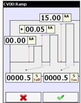
**HV Magnetization:** Similar test to the previously described, but using the Raptor HV, for the CT magnetization curve and knee point. Besides the capacity to use up to 2000 V, the connection is much simpler, simply connecting the voltage injection cables in the secondary of the transformer. Measurements during the voltage ramp injection are performed by the built-in ammeter and voltmeter of the HV unit.
