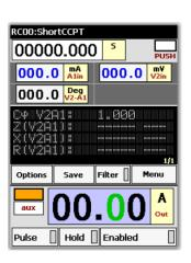
11. Voltage Transformer (VT): Checks VT turn ratio, polarity and primary/secondary phase angle, by applying voltage to the primary with the Raptor auxiliary voltage output, measuring the primary voltage with the voltmeter and the secondary voltage with the low signal voltmeter.
