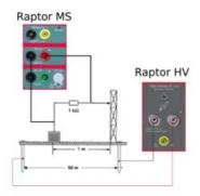
Touch voltage: The measurement is performed between an earthed accessible metal part and ground as shown on Fig.
