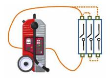
**3. Overcurrent Relay:** Through injection of a fault current through the primary of the CT, check correct operation of the protection, the effective trip of the breaker, and verify the complete primary/secondary/primary loop.
