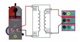
**19. HV PT short-circuit:** Using the HV, template to carry out short-circuited impedance tests in distribution and power transformers.
