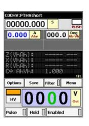
**17. HV Voltage Transformer:** Using the high voltage ouput of the HV unit, checks VT turn ratio, polarity, primary/secondary phase angle, and burden by applying voltage to the primary, and measuring secondary voltage.
