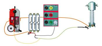
**9. CT Burden:** Burden connected must be lower than rated CT burden, and so this template enable us to determine if the CT is suitable or not for this burden. By injecting current through secondary, calculates impedance, power and power factor of the load. Current to be injected into the burden is the nominal secondary current of the CT, that is, either 1 A or 5 A.
