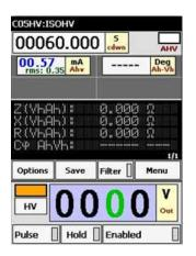
**16. HV Dielectric (Withstand Voltage Test):** used to check the insulation integrity of the transformer through the leakage current monitoring while injecting high voltage between primary and secondary, or between secondary winding and ground.
