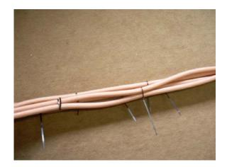
Even though tied, cables will try to separate from each other, and this must be avoided in next injections.
