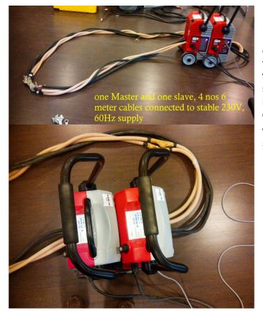
Here, the user nicely twisted the conductors to each other BEFORE threading them through the Raptor, which does not help eliminate the space inside the injection spire. As a result, the maximum current obtained was **1670 A only** (while with the proper cable layout up to 5500 A was possible)
