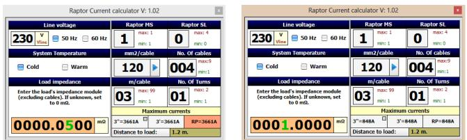
In the same way, the total test circuit impedance limits the current (load + cables + connections) so, using the shortest cables as possible has a direct impact on maximum possible current. The small size and weight of the Raptor allows placing it **closer to the device under test**, even to place the Raptor in a table, platform, raised close to the load, etc.., reducing the distance to the load, allowing using **shorter cables** and getting therefore higher current in the load.
