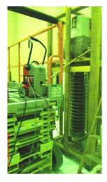
With the same purpose, it is placed more **cables in parallel** to reduce the impedance of the circuit. Sometimes the only solution to get the maximum current required is both, to reduce cables length and to increase cross-section of the test leads by adding cables in parallel (or using cables with bigger section).
