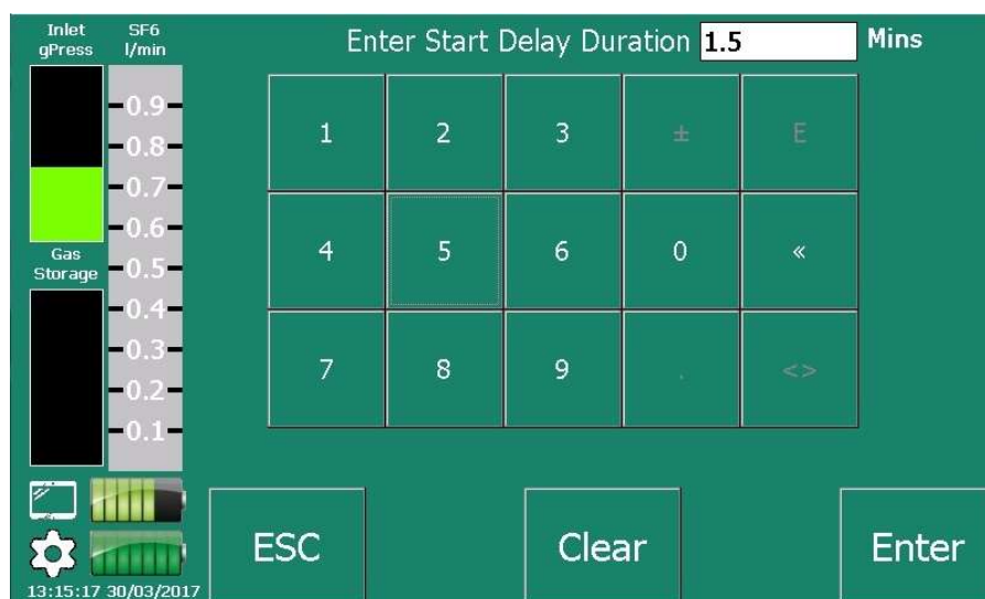
Figure 14: Enter a time up to ten minutes to use a delayed start
