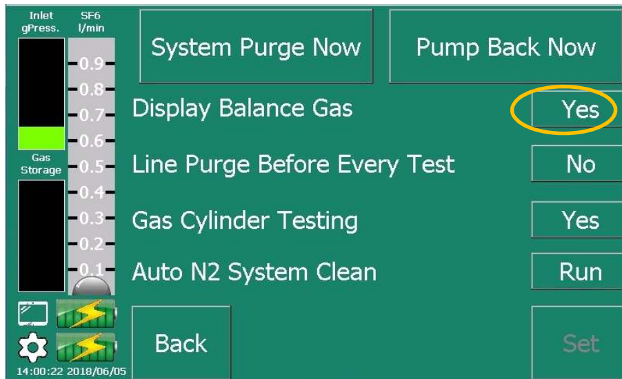
Figure 18: Use the System Control Menu to switch on / off the Balance Gas option
