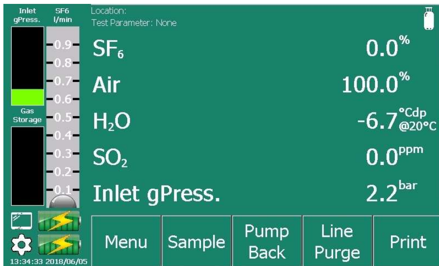
Figure 21: With Air selected as the unit for the balance gas, the display now looks like this.
