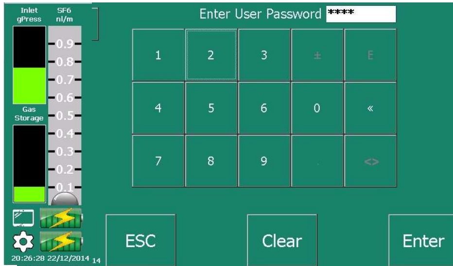
Figure 48: Once a password is enabled the user password will have to be entered to gain access to the menu button that is locked.
