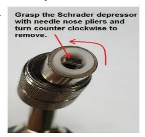
2 Remove and replace the Schrader depressor and/or the worn gasket.
