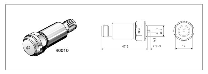
Glue-on transducers 40010 can replace standard transducers on thinwalled bearing housings and on machines where the drilling of standard mounting holes would affect equipment warranties. They have the same measuring characteristics as standard transducers, but a flat, circular base which is glued to the measuring point, and an M3 screw for unloading and fixing.
