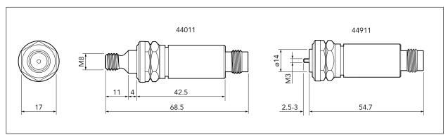
The 44000-family of transducers for potentially explosive atmospheres is approved for use in mining, explosive gases and dust.
