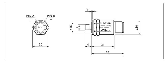
The vibration transducers series SLD300 are small accelerometers based on micro-electro-mechanical-systems (MEMS) technologies, designed for vibration monitoring of industrial machinery. The electrical signal is isolated from the transducer housing.
