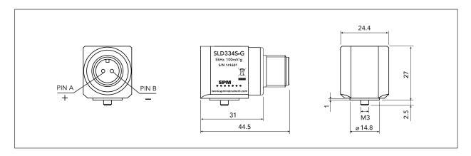
The glue-on vibration transducers SLD334S-G with side entry based on micro-electro-mechanical-systems (MEMS) technologies and can replace standard transducers on thinwalled bearing housings and on machines where the drilling of standard mounting holes would affect equipment warranties. It has a flat, circular base which is glued to the measuring point, and an M3 screw for unloading and fixing. The electrical signal is isolated from the transducer housing.
