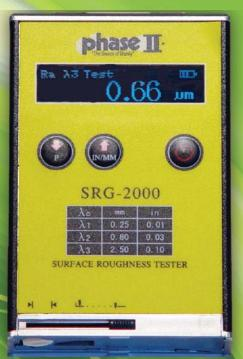
The SRG-2000 determines surface roughness parameters Ra,Rz, Rms(Rq) and Rt within a wide measuring range. The piezo-electric pick-up stylus with diamond tip assures a very reliable measurement within tolerances that conform to ASME B46.1. Surface Roughness parameter Ra is computed to conform to ISO and Rz is computed to conform to DIN.
