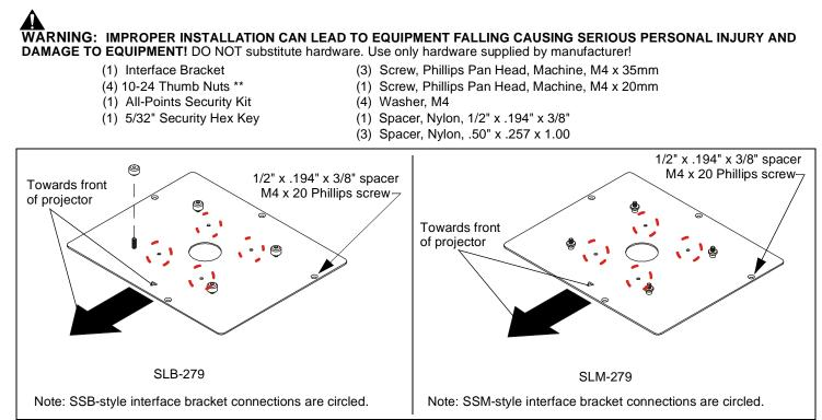
\*\*Only used when installing SLB/SSB interface brackets.
