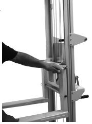
To invert the forks, remove the fork arms as described above. Rotate the fork 180 degrees and reinstall.
