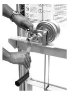
To reverse the winch handle, pull the spring loaded pin with one hand while sliding the handle off with the other hand. Rotate the handle 180° and reinstall. This places the winch handle in a secure location for transportation or storage.
