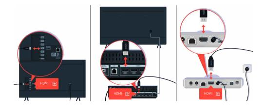
Check the antenna and HDMI cable connections.
