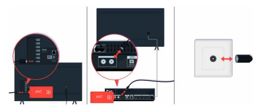
Check the antenna and input cable connections.
