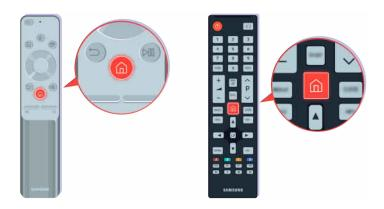
On the remote control, press the a button and move to  $\equiv$  Menu  $\Rightarrow$  a Settings  $\Rightarrow$  All Settings using the directional button.
