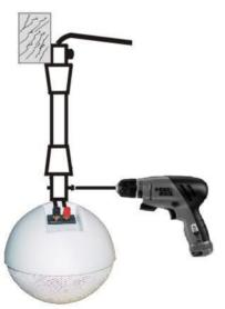
**6.** Insert pipe over the body stem of the Saturn speaker and add screw in with 1/4" x 20 screw.
