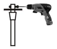
3. Screw in the nut and bolt into hade at the end of the pipe.
