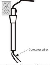
3. Run wire thru 1" pipe. Make sure you have enough to reach speaker terminal at the other end of the pipe.
