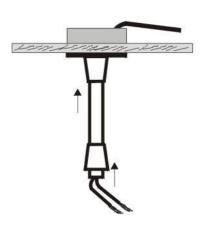
6. Slide the cap all the way to the metal plate and slide in the other cap at the other end pf the pipe.
