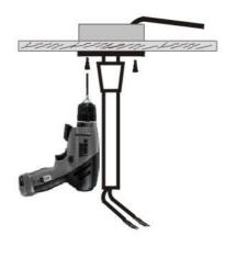
5. Screw the metal plate directly to the to the ceiling or to the gangbox.
