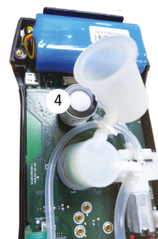
New sensor connected to electronic board
