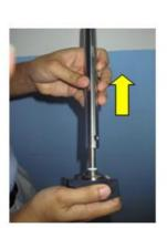
remove shaft tube and put it at a place where it cannot fall down as impact might damage it
