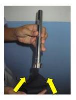
Use a piece of cloth to hold the stator as the teeth are sharp and can cut you!
