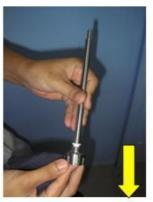
remove rotor stator and teflon bearing
