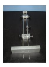
Once this bottom "H" has been fixed, take the double rod and insert into the middle piece of the foot stand. Turn it around and fix it with the other allen key using the smaller screws for it. Turn it around and fix the drive with the support rod at the upper boss head and the strap clamp at the lower boss head.
