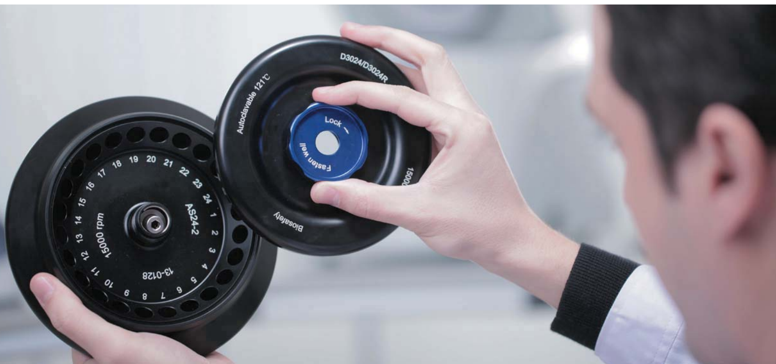
Seals within the aluminum alloy rotor
