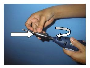
Put the shaft tube onto the axle and screw clockwise onto the housing!
