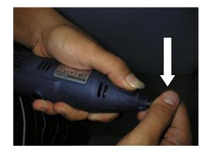
Hold D-160 drive open the collar and press the black button to lock it and unscrew the collar
