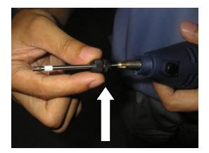
Put collar onto the shaft and screw it back to the drive itself! While doing that you must press the black button to lock it
