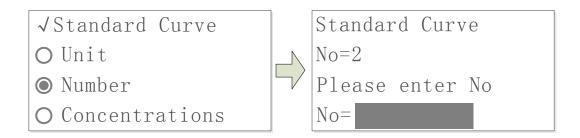
7) Calibrate Standard Samples. Put the corresponding standard samples in the light path as the screen indicates, input the concentration of the corresponding and press to measure.
