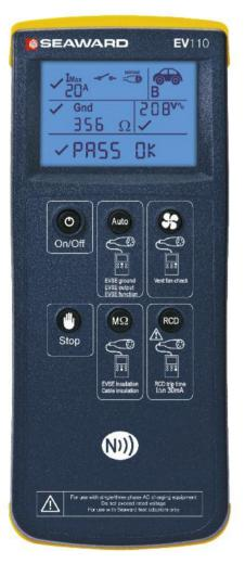
The EV110 is also able to simulate a number of vehicle faults, and automatically store the EVSE fault response including the disconnection time and the amplitude, frequency and duty cycle of the PWM communication between the EVSE and simulated EV.
