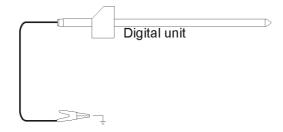
6.1.2 On connection of the insulated earth cable to the bottom of the handheld section the digital display is automatically powered up and zeroed ready for operation.
