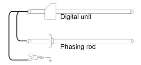
6.2.2 On connection of the insulated earth cable to the bottom of the handheld section the digital display is automatically powered up and zeroed ready for operation.
