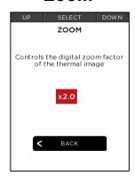
While imaging, press and hold the left button to continuously zoom up to 4X. You can also set the zoom factor manually in settings.
